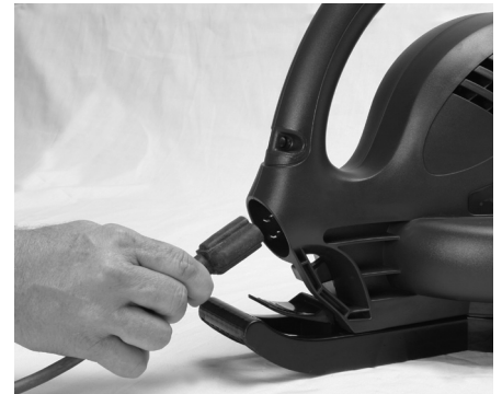
Figure 4-1: Plugging extension cord into inlet plug
